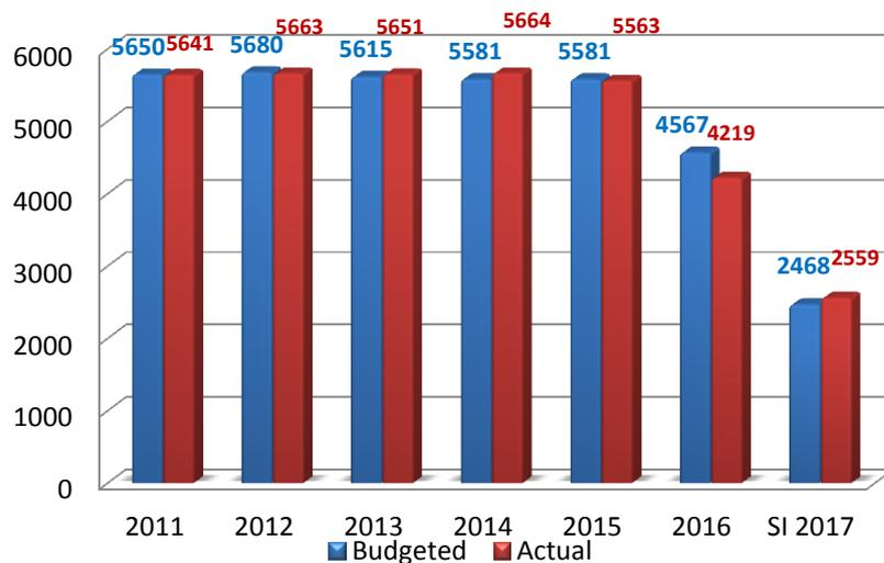
Analysis of the production data shows that the produced gas volumes were almost equal or exceeded the expected gas volume. The natural decline of the gas reservoirs was arrested in this period (average decline in the last years between 1-2% per year).
